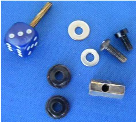
Pop a steel washer then a plastic, shouldered insulating washer on the screw & insert it through the top contact hole in the machine frame, followed by another plastic insulating washer, steel washer, front coil wire lug (maybe another washer), capacitor wire lug & another steel washer. DON'T do it all up real tight at the moment.
