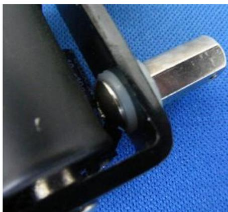
Now do the same procedure with the top binding post. Remove the contact screw from it first.
