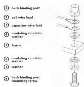
Horizontal back contact correctly fitted to machine.
