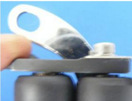
you're going to have to use a spacer under the back spring. Use a square steel spacer the same size as the width (front to back) of the spring saddle/back spring.
