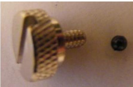
Carbon build up is common on the contact surface of the contact screw, so occasional filing or light sanding of the tip of the screw to remove the carbon build up is needed, but only remove the carbon build up, try not to remove too much metal from the screw,
