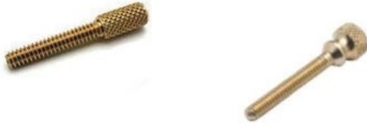
The point where the contact screw makes contact on the front spring will change a machine's performance. It's an important co-factor in the setting & adjusting of the distance the armature bar will travel (the stroke), by, among other things, acting as a limiter for the front spring, so it must be tightened or loosened in conjunction with the tension on the springs.
