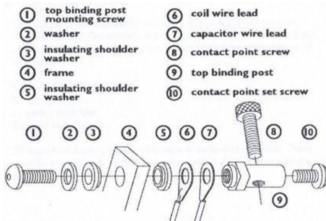
You can space out the top binding post from the frame with steel washers/shims to ensure the contact screw is positioned dead central to the middle of the front spring.
