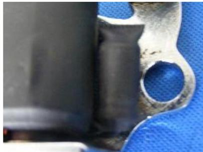
Loosen the coils again so you can tip them sideways a little & place the capacitor where you want it & do the coil screws up again. Check the capacitor isn't being squashed or any of its wires, or the coil wires, anywhere. If it's all good...do the coil screws up good & tight now.
