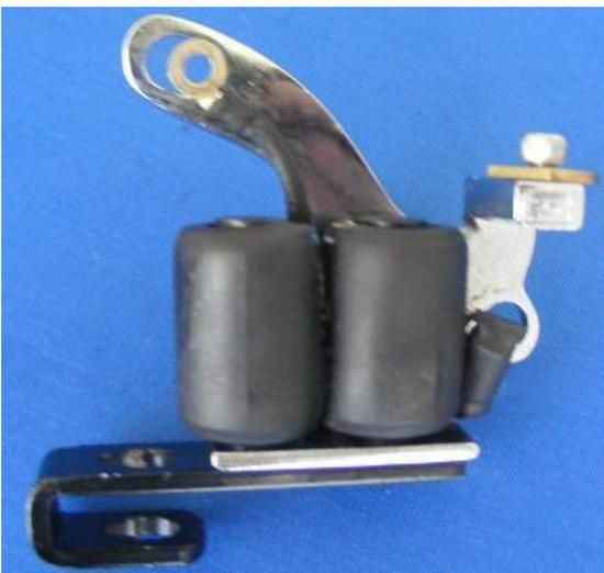
Attach the armature bar/back spring to the spring saddle, lining it up straight over the coil
