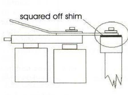
Then go through the coil height routine again...the front coil will need shimming to give it a slightly higher profile to the rear.
