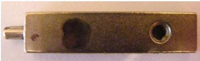
Always try to replace the armature bar in the same position on the machine, mark it in relation to the front coil core with a small dot of Tipex
