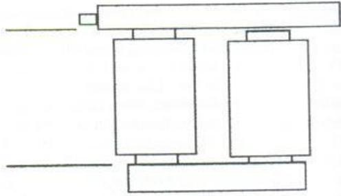
If it deflects downwards even the slightest bit, you're going to have to shim up the front coil. Same deal if it touches BOTH coil tops, it doesn't want to be touching the back coil.
