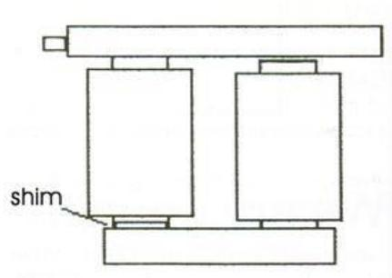
Then with the armature bar pressed down on the front coil, look at it from the front of the machine, checking the bar sits flat & square to the top of the coil...
