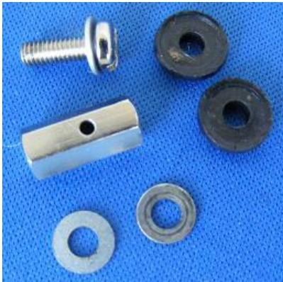
On a sideplate style frame, hold the machine with the back of the machine towards you, pop a steel washer & then a plastic insulating washer on the screw & place it in the back contact hole in the frame, then on goes the other plastic insulating washer, a steel washer, the soldered lug from the back coil, the soldered lug from the capacitor & another steel washer. Depending on the neatness of the soldering/thickness of the insulation on the lugs, you might well need a washer between them, too.
