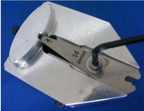
The armature bar alignment tool.
