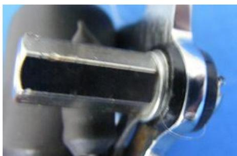
The only time your going to have a sight problem is if the fitment on your frame fits horizontal through the rear upright of the frame....in that case, fit the binding post BEFORE the rear coil....otherwise you wont be able to get to the screw head....it'll be 'hidden' by the rear coil! It'll take a bit of juggling with the coil/wires/capacitor etc., like the machine in the picture below.
