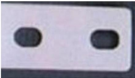
The benefit of this is that they will fit in exactly the same way, every time. The drawback is that the whole front/back spring/armature bar/securing screw/washers have to be completely disassembled & reassembled, every time you want to change a spring, which is a complete nightmare when your setting up/fine tuning a machine or experimenting with various spring gauges!
