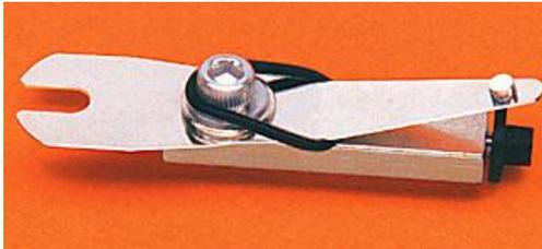
The front spring establishes the speed that the machine will run & the back spring determines the efficiency of the front spring. The action of one spring will be balanced by the other, the result being measurable as a correct duty cycle.
